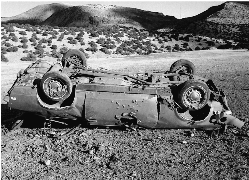
FIG. 6—Post-blast damage to vehicle at 4.6 m.
