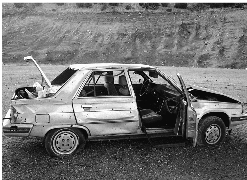
FIG. 8—Post-blast damage to vehicle at 22.9 m.
