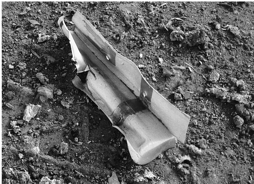
FIG. 3— Post-blast damage to sign at 7.6 m.
