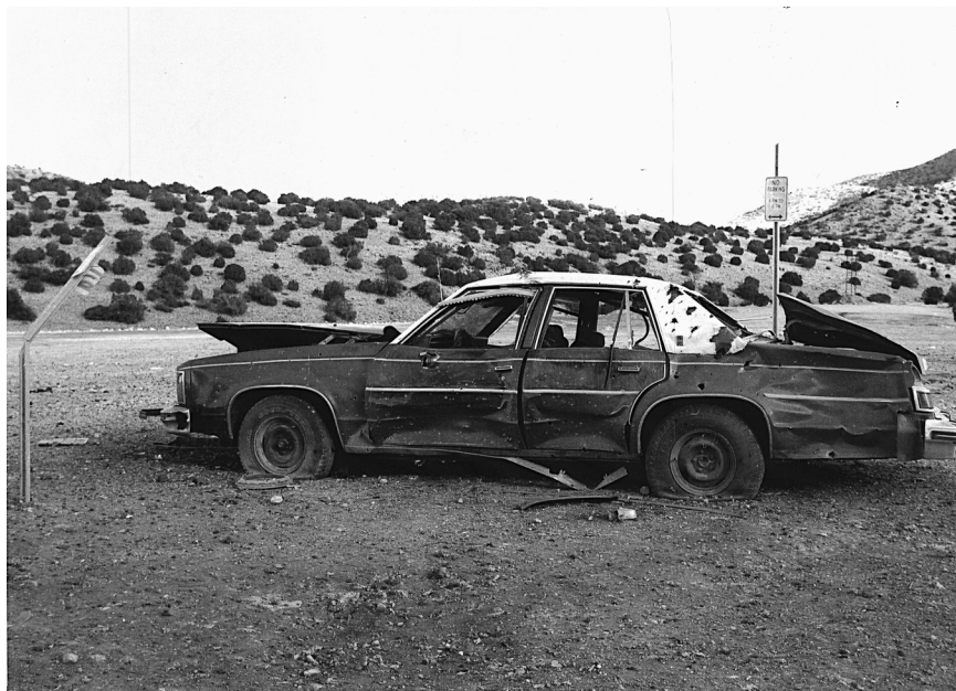
FIG. 7—Post-blast damage to vehicle at 15.2 m.
