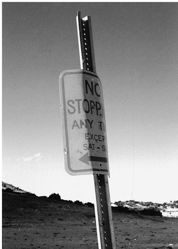
FIG. 4—Post-blast damage to sign at 22.9 m.
